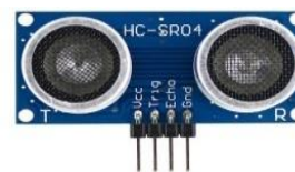
Fig.2. An ultrasonic sensor
